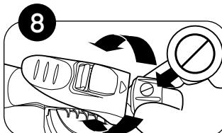
When not in use rotate control knob to OFF position. To prevent leakage, always store and use the bottle in an upright position. Turn off and disconnect from water supply after use.
