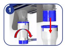
Disconnect the Safepack connector(s) by turning from the product pouch
