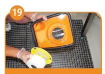
Uncouple the recovery tank cover from the hoses and detach the floating unit.
