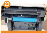
Clean brush housing after work process and check periodically the valve and the fresh water filter.
