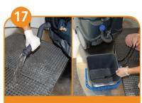
Empty fresh water into a sink through the blue marked draining hose or into a bucket by using the additional draining hose.
