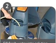
Fill fresh water into solution tank with a coupling hose or by using a bucket.
