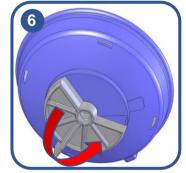
Check the rotating part of the powder cartridge(s) by moving the rotor through 360°
