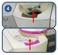
Check the feeder inlet(s) on liquid residues and/or incrustation/clogging
