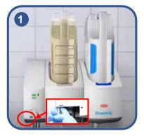
Switch off the dosing system by pressing the ON/OFF switch
