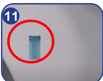
Fully push in the dispensing button once and wait ensuring the sight glass is full of product.
