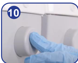
Fully push in the dispensing button once and wait ensuring the sight glass is full of product.
