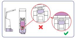
Ensure pouch is seated correctly. Apply downward pressure until  $\alpha$  'click' is heard. If pouch is seated incorrectly, Dispensing Button (1) may not return to original position.
