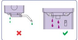
Check product is not leaking from the Delivery Spout (5) or Overflow Drain (6). If product is leaking from the Overflow Drain (6), remove and inspect Product Pouch (7) for splits.
