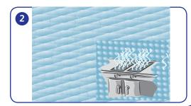
After cooling and draining, scrub remaining residues from side walls and heating elements with a scourer or brush. Rinse twice with clean, hot water and allow to air dry.
