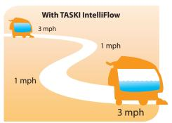
Without TASKI IntelliFlow, solution is delivered unevenly. As the machine slows in turns, more solution is released per square foot, causing puddles, wasted supplies and more frequent tank refills.
